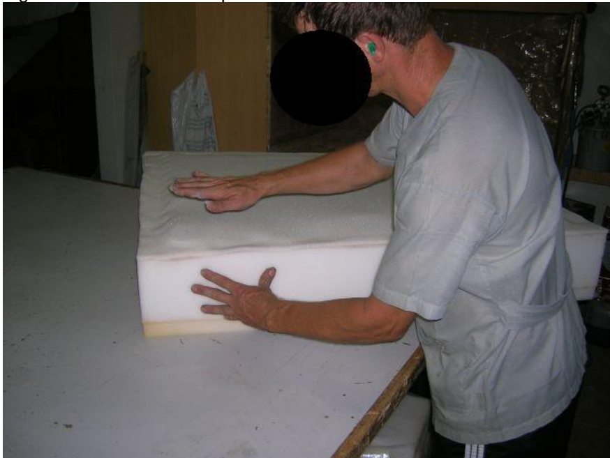
Figura 20 – Colando as espumas
